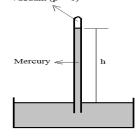
**2-** The pressure of water in a pipe is measured by a mercury simple manometer, as shown in figure.
